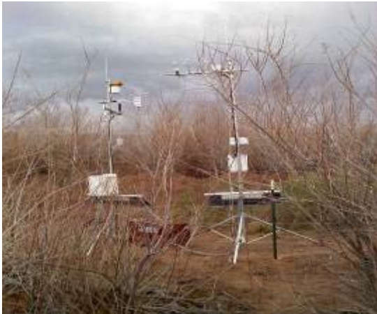
Figure A3.1. Photo of Eddy Covariance set up in February of 2010.
