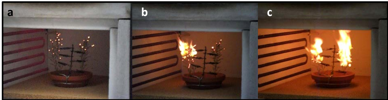
Figure III.5. Foliar flammability apparatus composed of alligator clips, stainless steel wire, secured to a 10 cm terra cotta tray. Glowing or charring is shown in a, flaming is shown in b, and consumption is shown in c.
